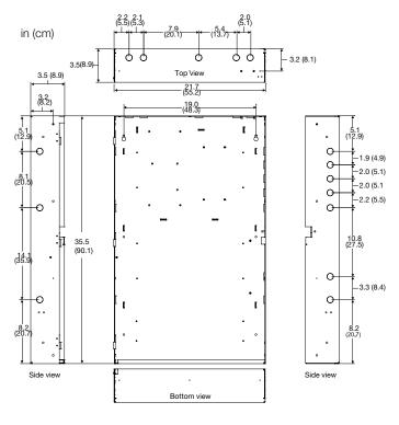
**Note:** Add 0.25 in (0.64 cm). to height and width dimensions to allow for knockouts when framing in the backbox for semiflush mounting.
